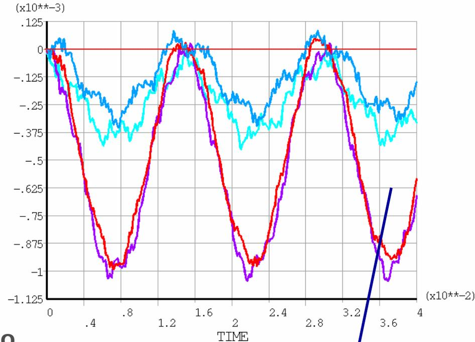
The displacement pattern seems to be the same as for simplified model, with a non-uniformity in z ... unfortunately the drift is much slower  $\Rightarrow$  longer analysis time!!
