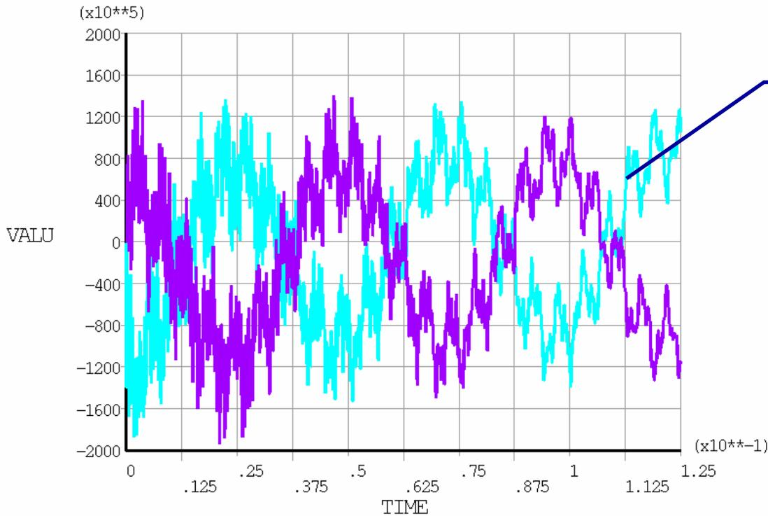
Bending stress at mid-span on Cu-strip face
