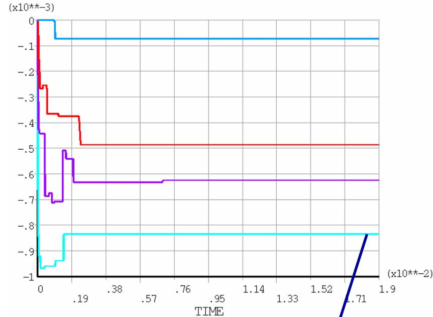
Longitudinal strains are always negative and seem to have stabilized after some millisec.
