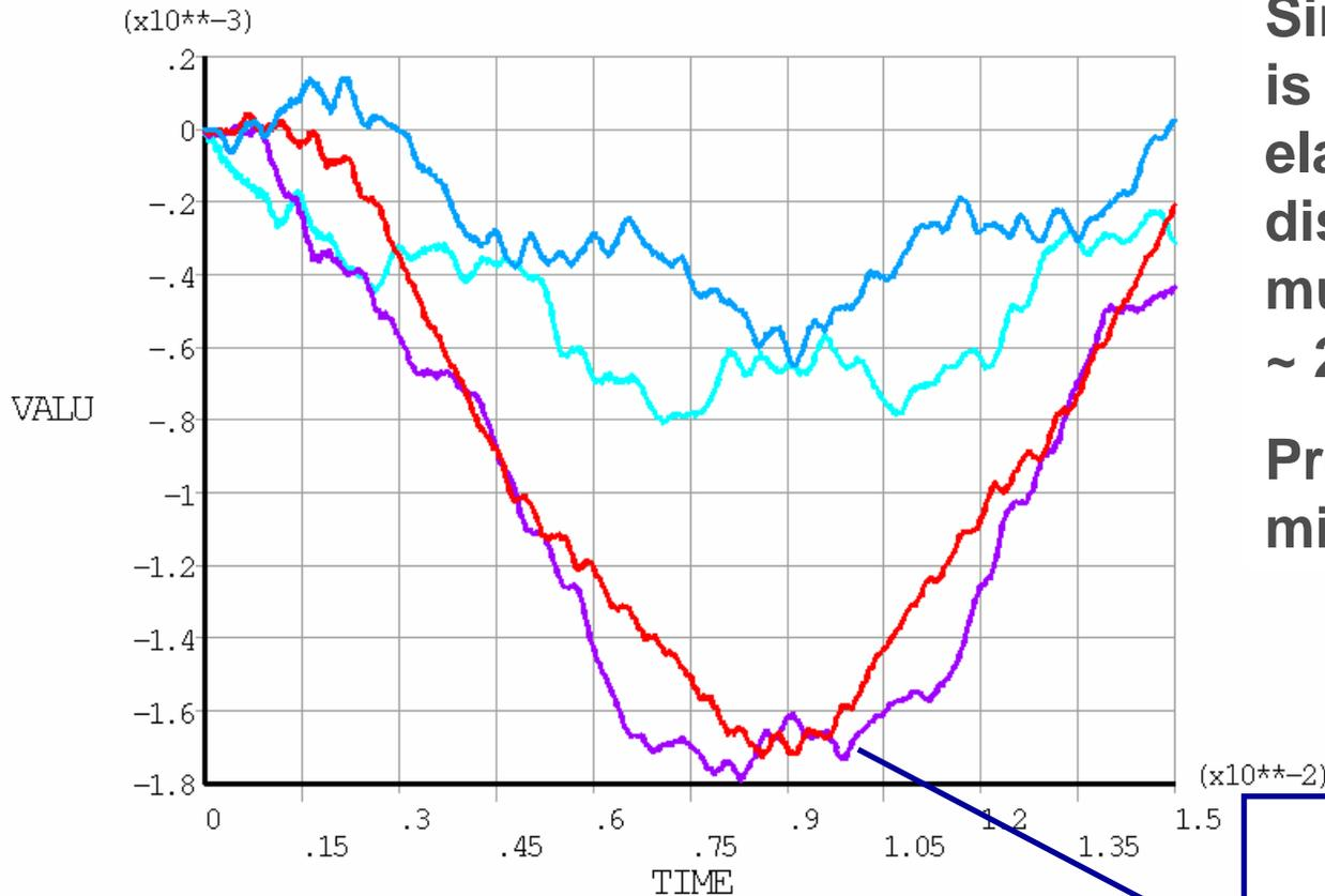
Since the behavior is almost fully elastic, displacements are much larger  $\Rightarrow$  up to  $\sim 2\text{mm}$  at jaw center.
