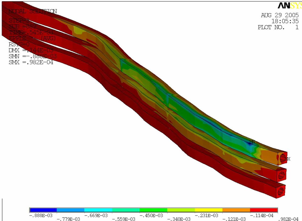
A certain degree of plasticization is found also on pipes (though here in Cu-OFE) ⇒
