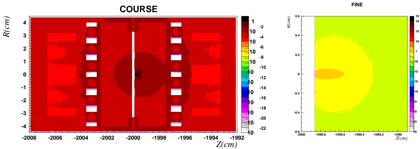
XY sectional views of raw fluka output (GeV/cm<sup>3</sup> per p<sup>+</sup>)
