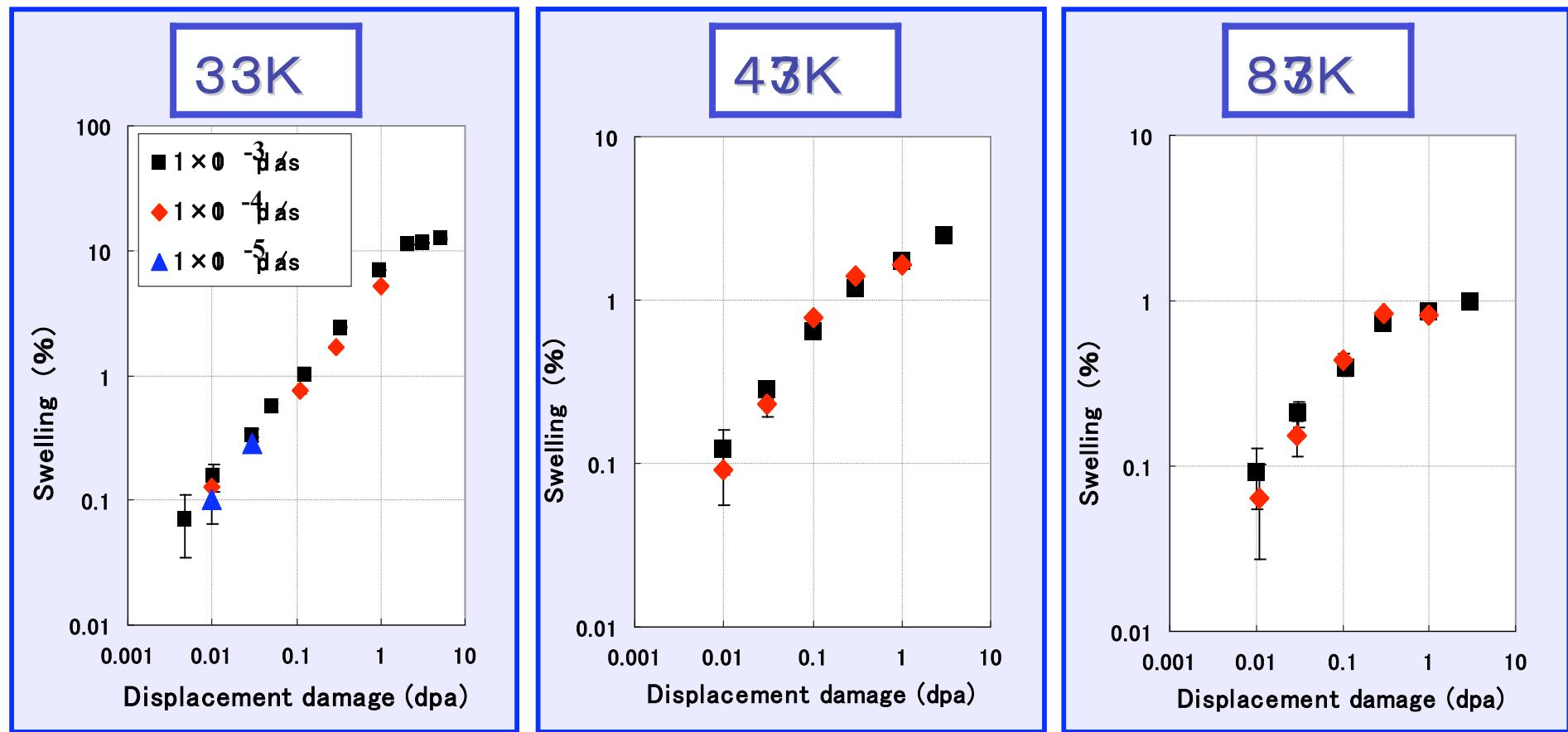
The displacement damage rates were  $1 \times 10^{-4}$  and  $1 \times 10^{-3}$  dpa/s at 333K-873K and  $1 \times 10^{-5}$  dpa/s at 333K with single-beam irradiation. The error bars represent the 96% confidence limits for the Gaussian distribution.
