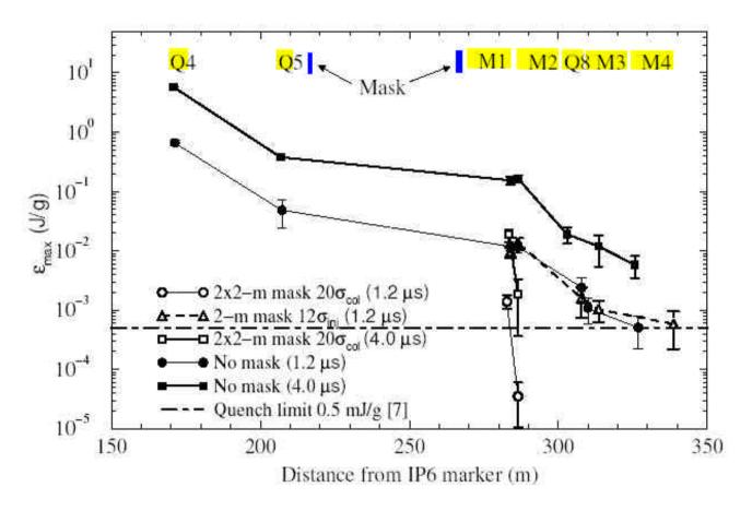
Two additional masks limit the quench region to one dipole with other magnets downstream remaining superconducting. Unfortunately, the masks need to be closed to  $20\sigma$  at 7TeV, i.e. they need to be movable... so forget it for the moment.
