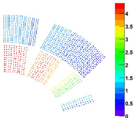
Temperature in the coil at I=7300A,  $\Delta T_{\text{simulation}}$
