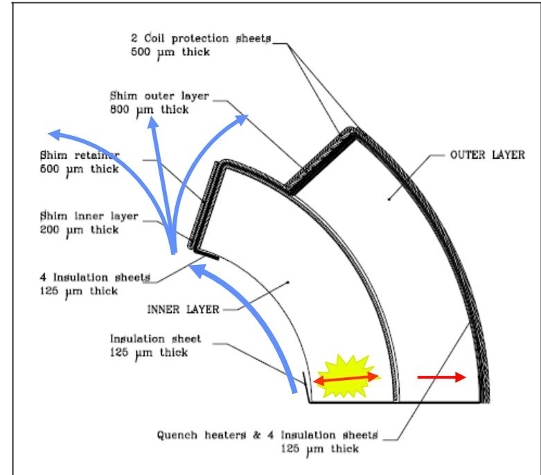
A heat transfer in the main dipole. Arrows indicate the radial path of the heat transfer in the magnet.
