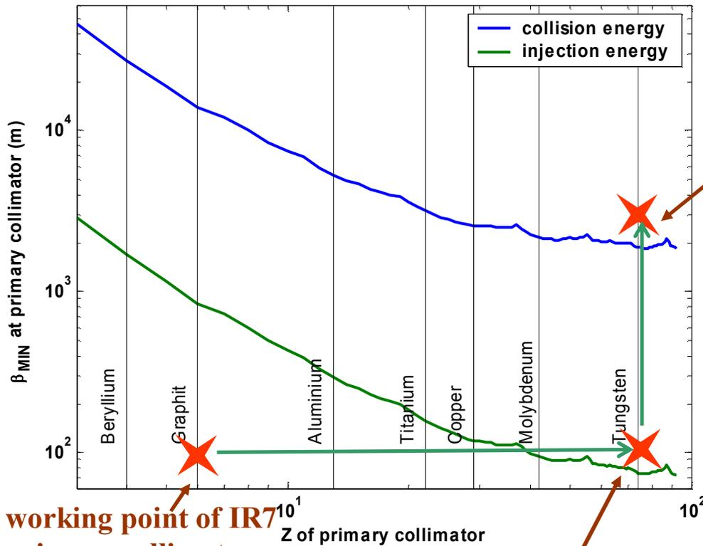
working point of IR7 primary collimators for protons
