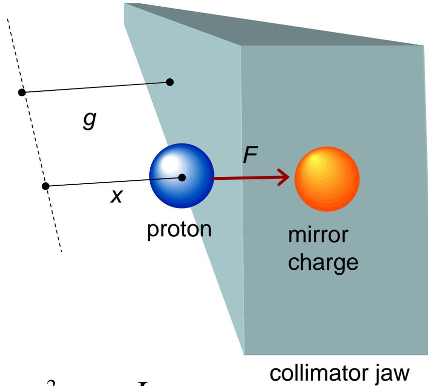
$$\delta x' = \frac{e^2}{16\pi\epsilon_0 m_U c^2} \frac{Z^2}{A} \frac{L_{\text{jaw}}}{(\beta\gamma)^2 (g-x)^2}$$
