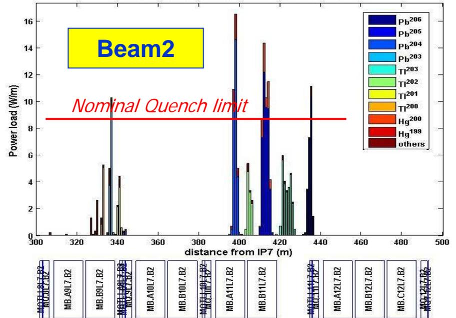
Beam 2 @ collision Particle losses in IR7,  $\tau=12\text{min}$
