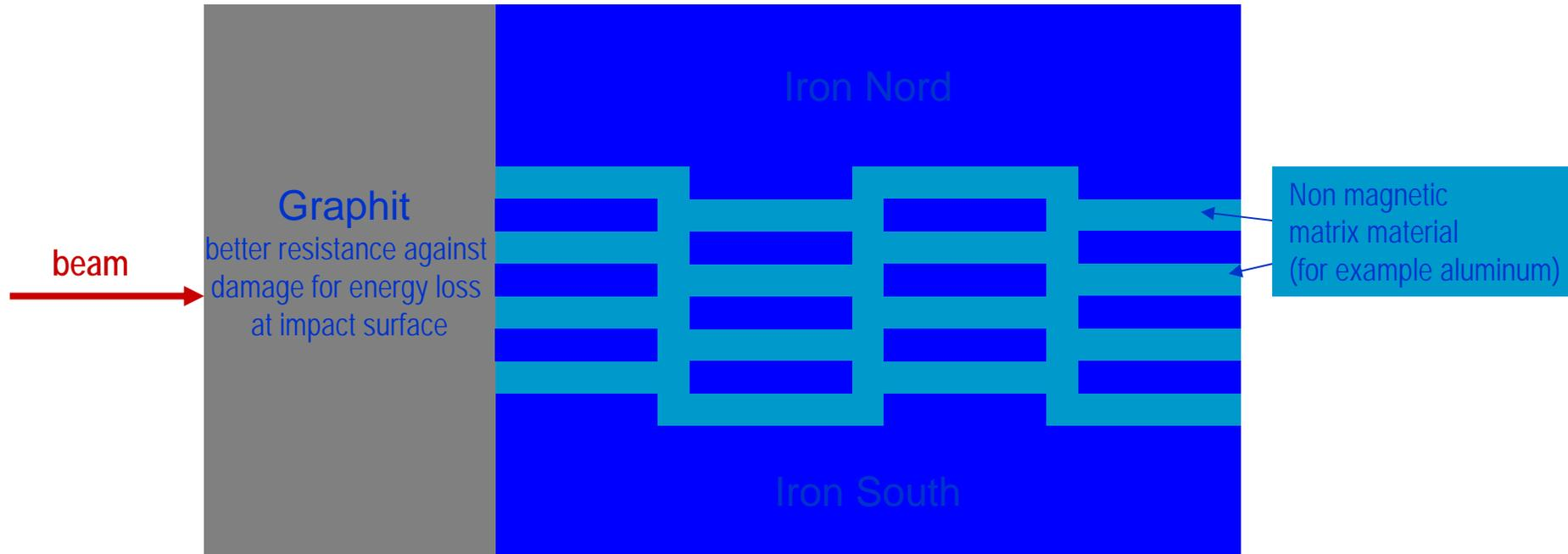
Interleaved positioning to cover all initial  $y$  positions
