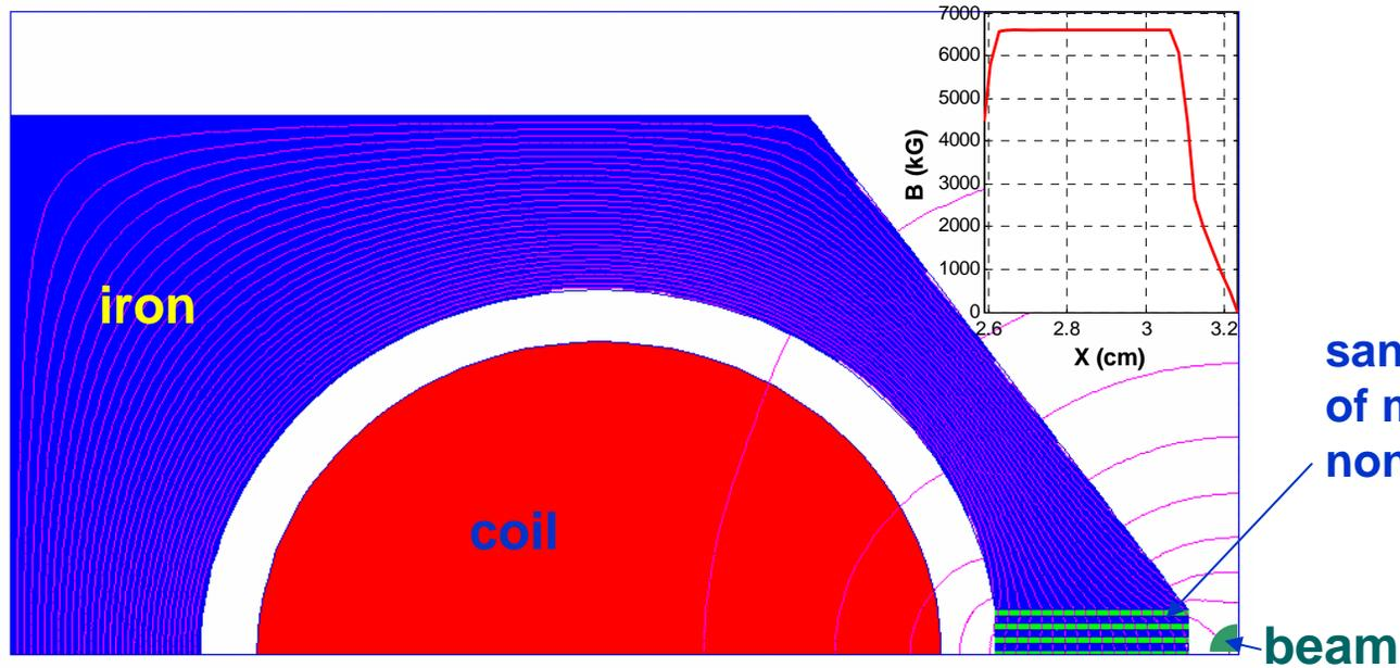
sandwich structure of magnetic and non-magnetic metal
