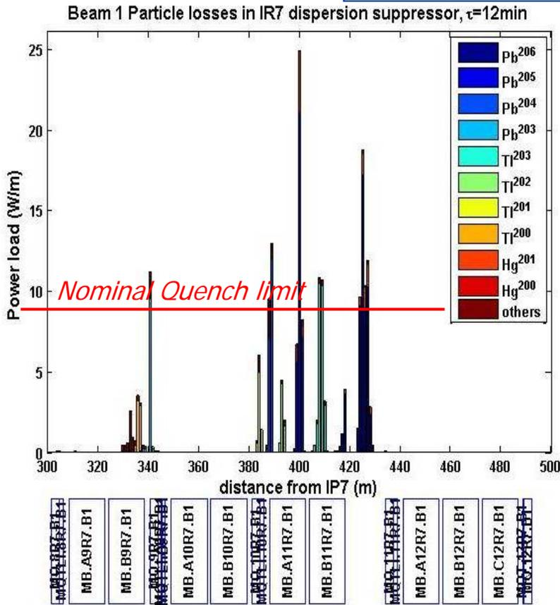
Losses confined to IR7 dispersion suppressor, cells 9 & 11
