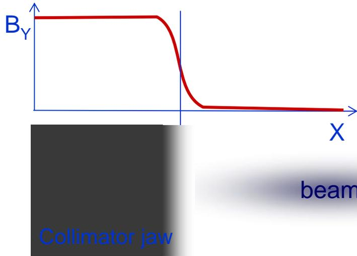
Condition to bend particle sufficiently to hit secondary collimator
