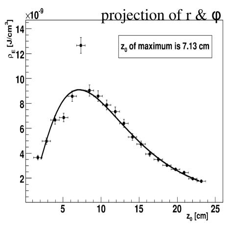
$\rho$ =k[wt<sup>a-1</sup>exp(-bt)+(1-w)l<sup>c-1</sup>exp(-dl)] w-"electromagneticity" of the cascade
