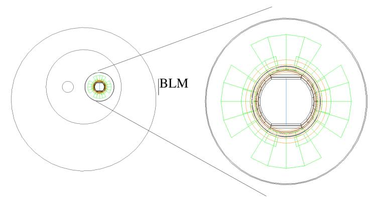
Coils are divided into small cells in (in  $r, \phi, z$ ) which energy is measured.
