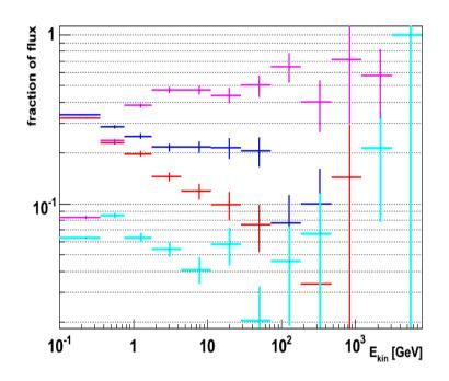
Origin: there are almost no particles directly from the wire; impacting angle of the most energetic particles corresponds to locations on the beam screen of D4
