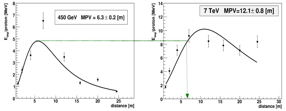
Signal in PMT scales with energy deposited in scintillators – there is a lot of signal at nominal luminosity – maximum 6-12 meters from WS, the signal level at
