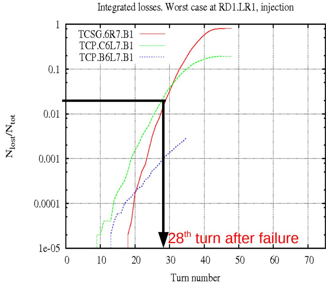
Knowing that 4 turns are needed to dump the beam (RS01 and RS02) therefore the threshold should correspond to loss during 24<sup>th</sup> turn.
