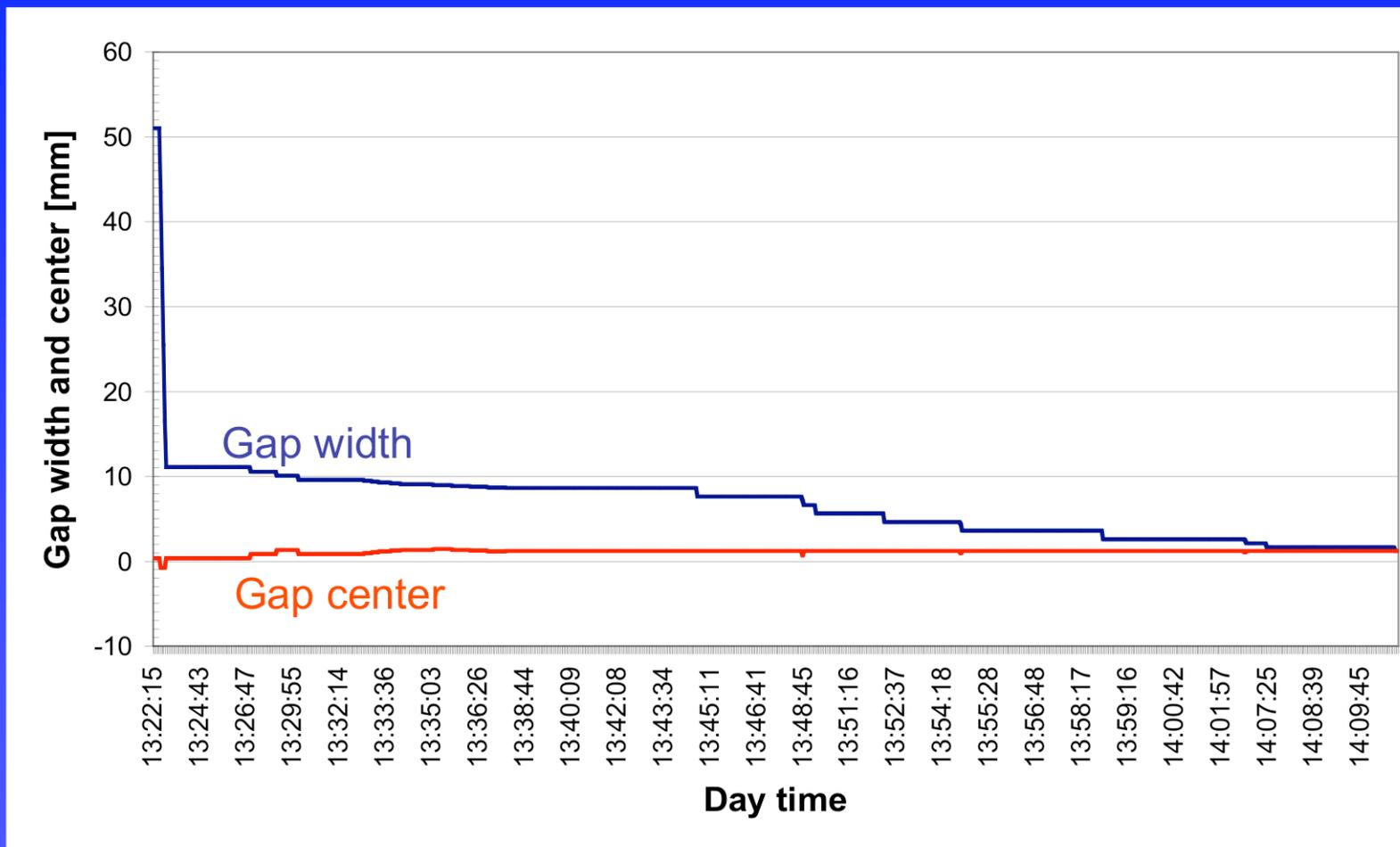
Down to 1 mm with stored beam → **Gaps smaller than required in LHC achieved!**
