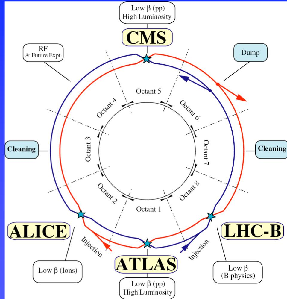
→ Four collimation systems: Momentum and betatron for two beams!
