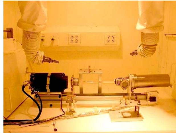
**Dilatometer Set-up In Hot Cell #1**
