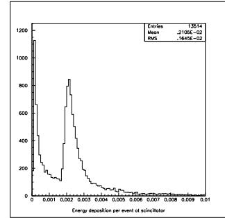
Figure 7: The analog spectrum in the scintillator as simulated with GEANT.
