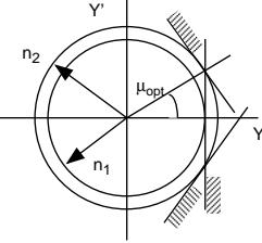
Figure 3: One dimensional betatronic collimation. A particle is scattered close to its maximum transverse position  $Z = n_1$ . If it is not absorbed, it is scattered along the vertical line  $Z = n_1$ . If a secondary collimator is at the depth  $n_2$ , the shortest cut along this line is made with a secondary collimator at the phase advance  $\mu_{opt}$ .
