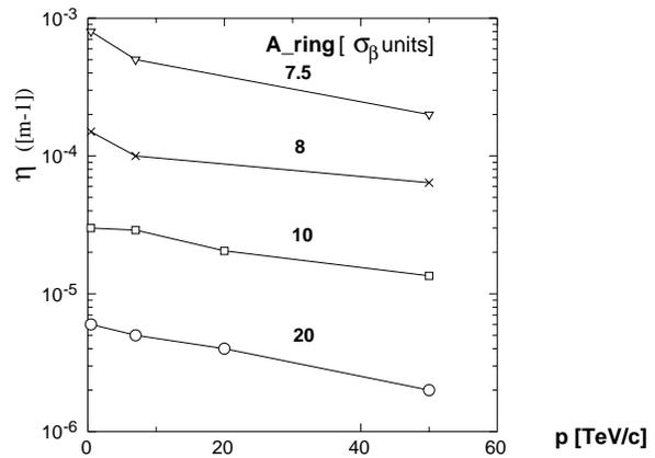
**FIGURE 2.** The inefficiency  $\eta$  of a two-stage betatron collimation system simulated with K2 for different beam momenta. Here three primary collimators are used (delimiting an octagonal normalised aperture, with primary and secondary retraction of the jaws  $n_1 = 6$  and  $n_2 = 7$  respectively).
