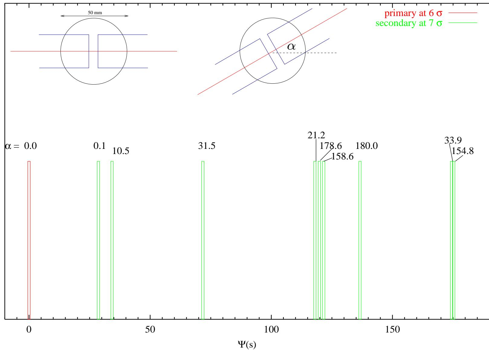
y-axis: number of MBs which would cause a closed orbit displacement of  $n \cdot \sigma$  (x-axis) at the collimator during a quench; no collimator at 90° phase advance from the primary
