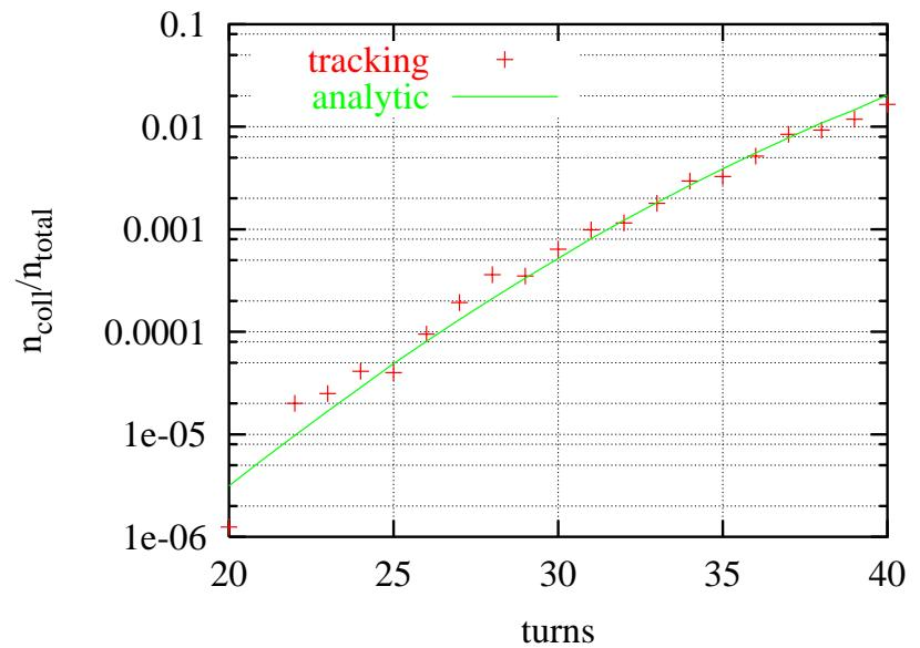
D1 magnets at IP1 and IP5, prim. collimator in IR7 ( $6\sigma$ ): Total number of particles at the collimator relativ to initial number of particles in the ring
