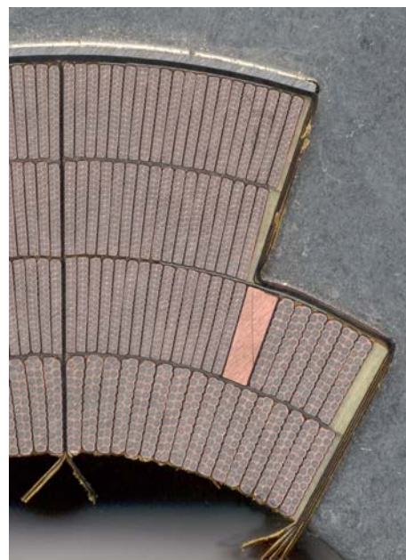
Photo of the MQY magnet cross-section
