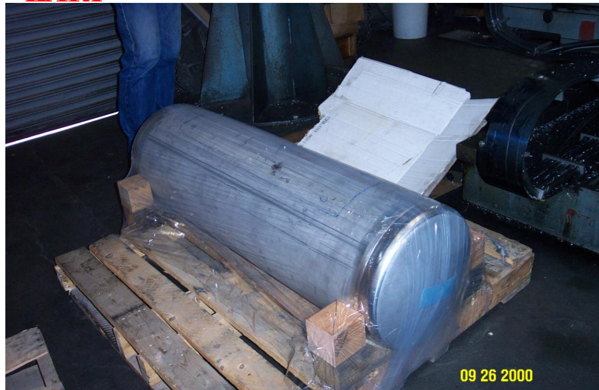
Vacuum chamber welded up
