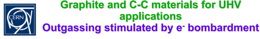
Sample: 14 cm<sup>2</sup> Heating power: 175 W (2.5 keV, 70 mA) Bombardment duration: 3 min. Temperature reached: 1050°C Effective pumping speed: 40 l/s
