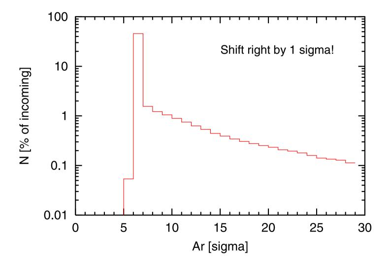
Not much shadow! Downstream collimators will be hit by ~50% of perturbed beam!
