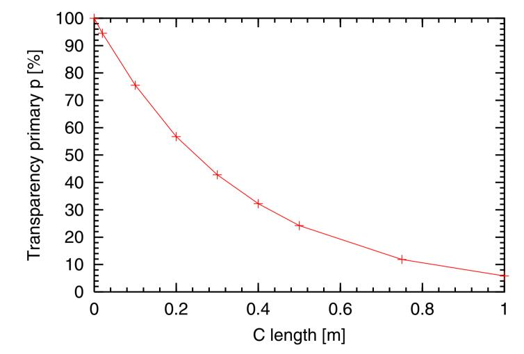
Primary 20 cm C collimators leak 60% of primary beam...
