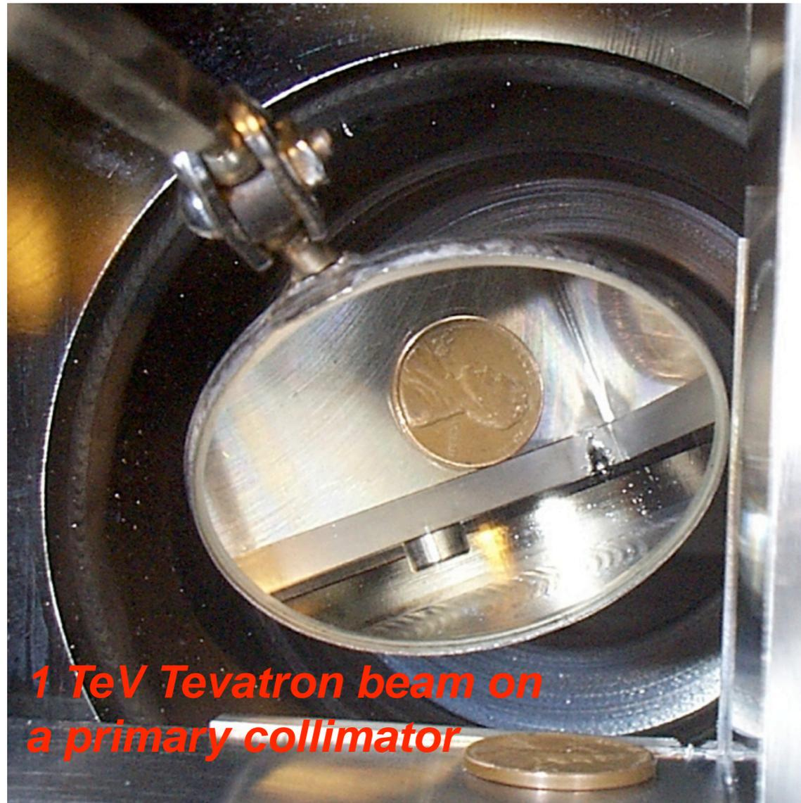
**1 TeV Tevatron beam on a primary collimator**
