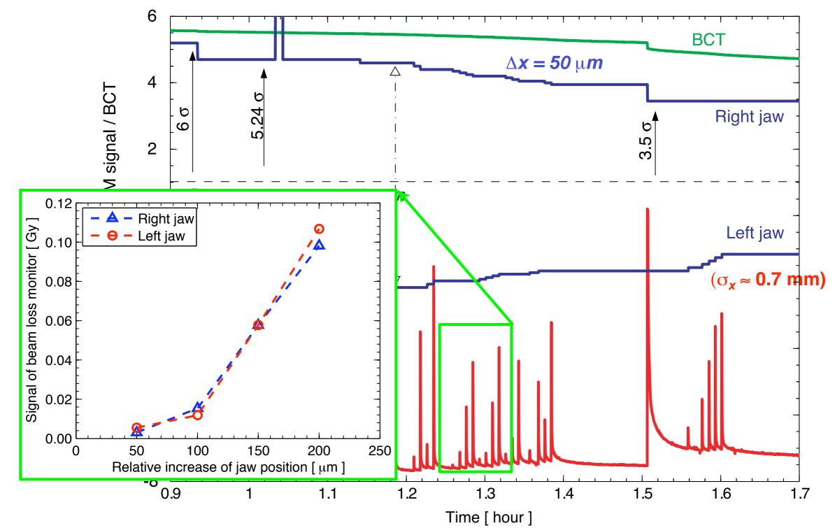
First centering with high-intensity beams: 1h. **50**  $\mu$ m centering accuracy demonstrated! Then, 10-15 minute (precision of 50  $\mu$ m). Less time for less precise settings. Setting of gap values relied on good optics model + emittance measurements.
