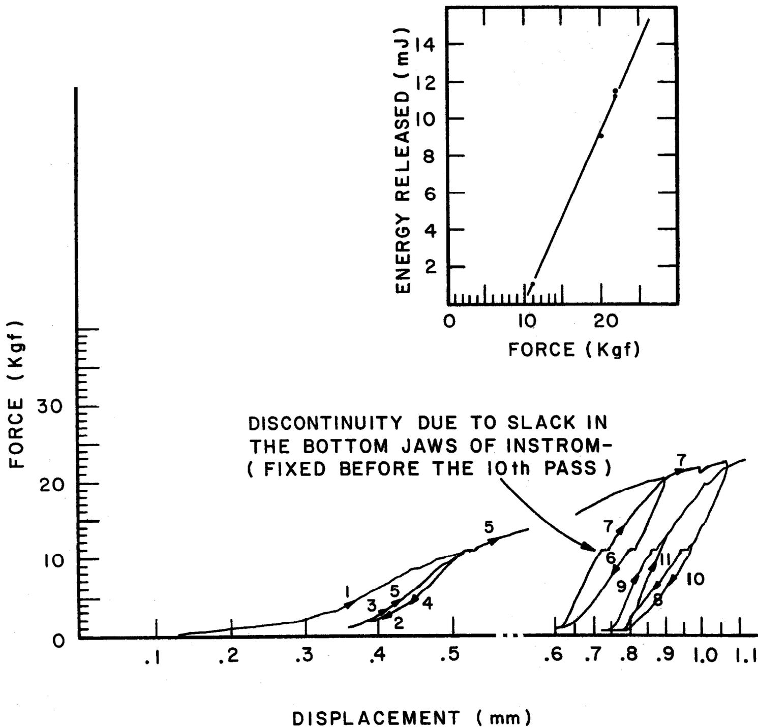
FIGURE 4 ROOM TEMPERATURE INSTRON TEST ON MULTIFILAMENTARY NbTi-Cu WIRE
