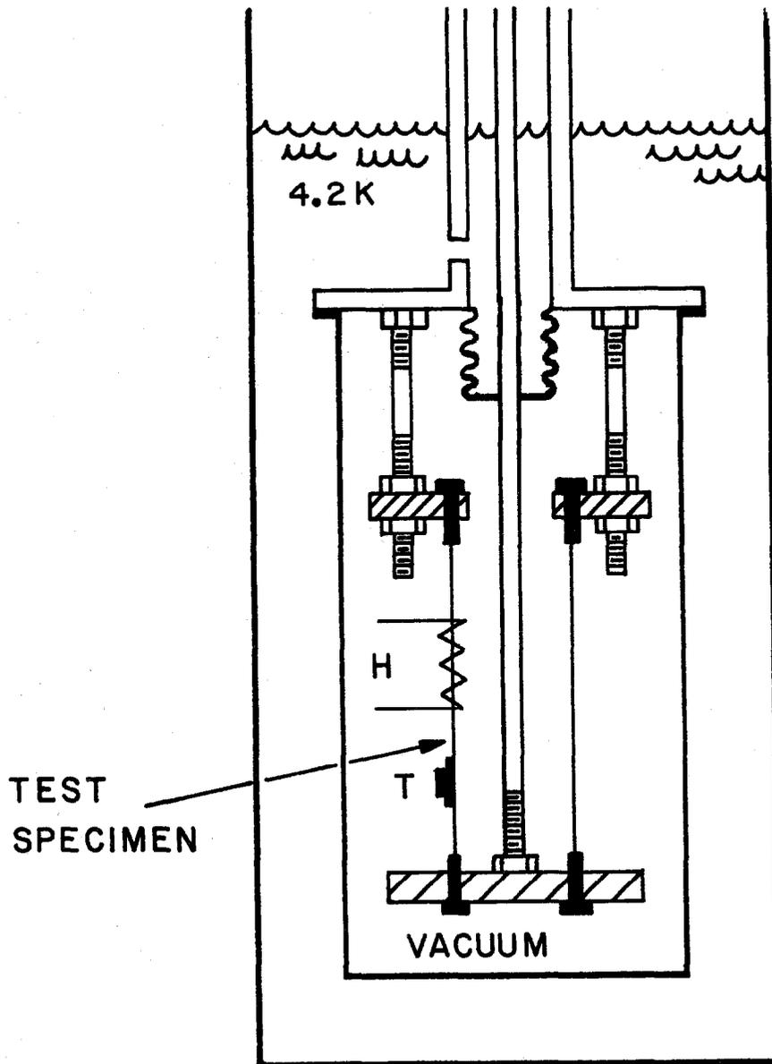
FIGURE 1. SCHEMATIC OF THE TEST SET-UP SHOWING THE HEATER, H, AND THERMOMETER,
