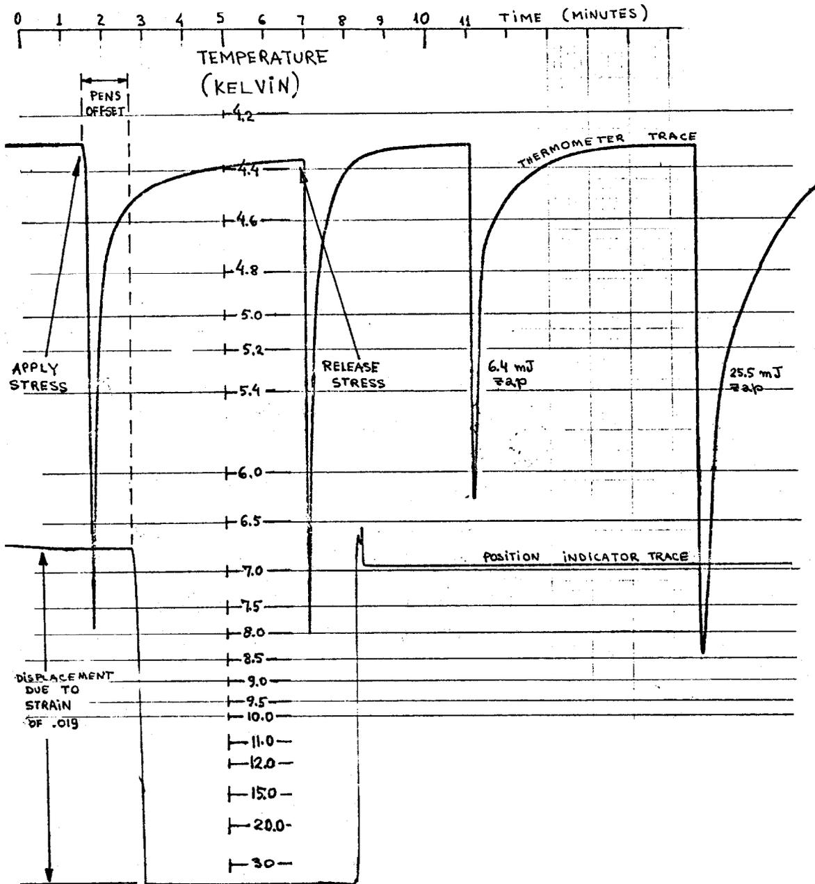
FIGURE 3. CHART RECORDER TRACES OF THE THERMOMETER (UPPER TRACE) SHOWING AN APPLICATION AND RELEASE OF  $153 \times 10^3$  PSI STRESS FOLLOWED BY TWO CAPACITOR DISCHARGES. THE LOWER TRACE IS DISPLACED TO THE RIGHT AND RECORDS THE POSITION OF THE STRESS APPLYING MEMBER.
