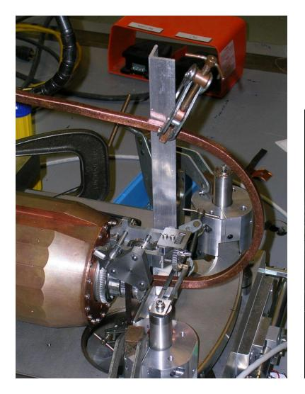
Rotate several facets while twisting Cu tube (note it is clamped in L photo) Ceramic race on one of the two bearings on actuator fails under load
