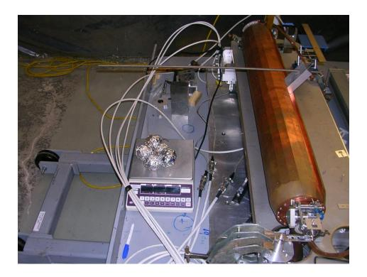
Lever arm (16") and weights (13.36 lbs.) with scale provides measurable torque for systematic studies
