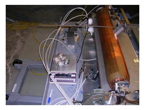
Setup to apply arbitrarily large torque to test rotation drive at many time expected torque required
