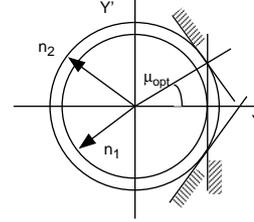
Figure 3: One dimensional betatronic collimation. A particle is scattered close to its maximum transverse position  $Z = n_1$ . If it is not absorbed, it is scattered along the vertical line  $Z = n_1$ . If a secondary collimator is at the depth  $n_2$ , the shortest cut along this line is made with a secondary collimator at the phase advance  $\mu_{opt}$ .
