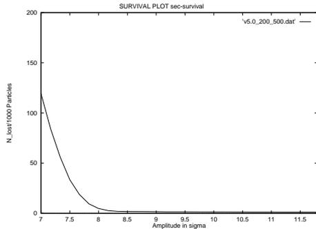
Figure 5: The survival plot in LHC at injection with the cleaning insertion described above, see text. In abscissa, the radial betatronic amplitude  $A_r$ . In ordinate, the function  $F_s(A_r)$ , normalised to 1000 events touching a primary collimator. See text.
