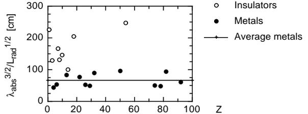
Figure 2: The reduced length  $\lambda_{red}$  as a function of the atomic number  $Z$ . For metals (black dots),  $\lambda_{red}$  is nearly constant with an mean value  $\lambda_{red} = 0.66$  m and a relative variance  $\sigma(\lambda_{red})/\lambda_{red} = 0.3$ .
