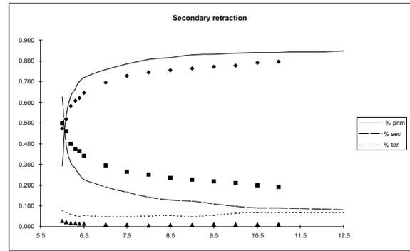
Figure 8: The raw relative rates measured at the collimators. Diamonds and upper curve: PRIM, squares and medium curve: SEC, triangles and lower curve: TER. Points are raw measurements (for some corrections see text). The curves are the result of multi-turn tracking and scattering in jaws made with the K2 code. The wavy structures on the curves are of statistical nature. The data analysis is preliminary.
