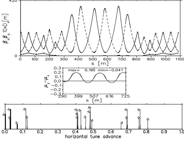
Figure 4: IR7 lattice and tune-split functions for LHC version 5.0, with the IR7 quadrupoles tuned for high positive tune split, giving  $A_{max} = 8.45\sigma$ . The range of tune advance (in  $2\pi$  units) corresponds to the range  $s \in [290, 725]$ .
