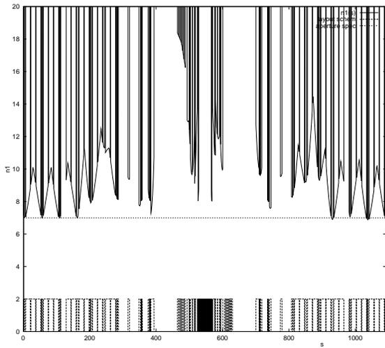
**FIGURE 1.** The normalised aperture of the insertion 1 of LHC after matching with aperture constraints, expressed in terms of equivalent primary aperture  $n_1(s)$ .
