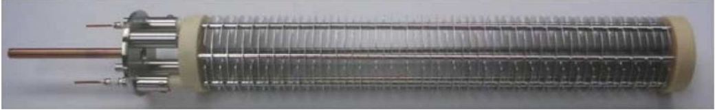
(a) A BLM ionization chamber without its casing
