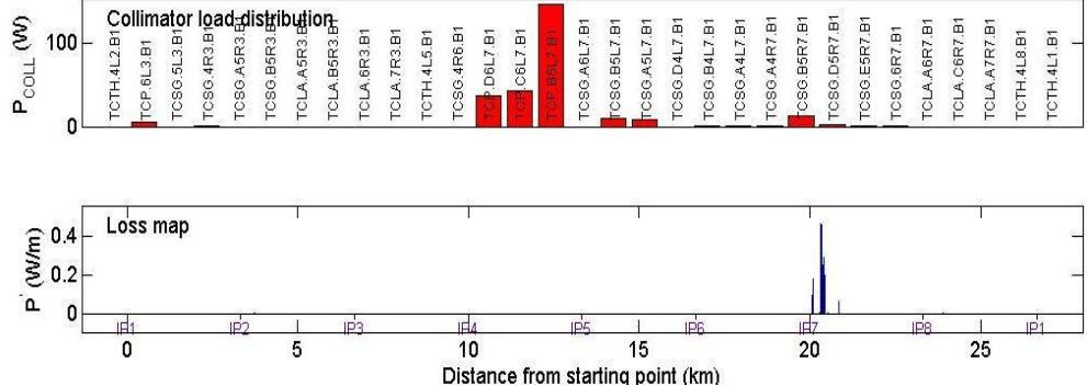
Max load on TCP.B6L7.B1=122W
