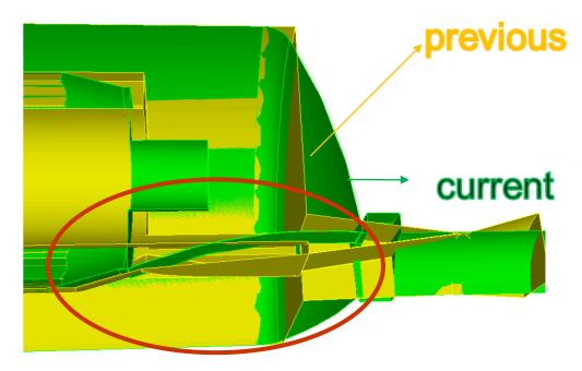
Narrow EM foils as well as large distance between EM foils cause more Ez fields existing in the end regions of the vacuum tank along the beam path.
